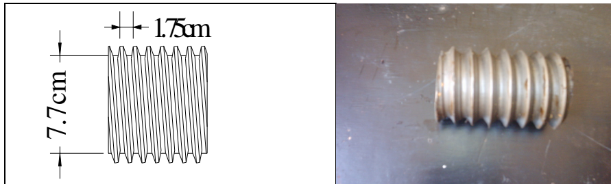
Fig. (8): The design of final screw design.
