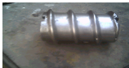
Fig.(5): A photo of the new feeding screw part.
