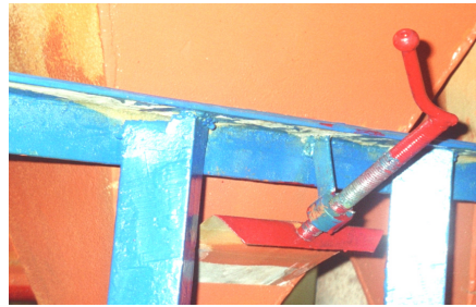
Fig. 4: The slide gate
