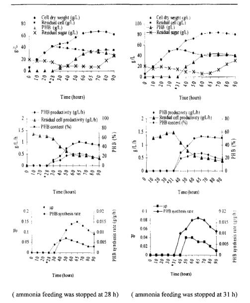
Fig.(3): Growth of *R.eutropha* ATCC 17697 and PHB production during 90 h incubation at 30°C on med.3 under nitrogen limitation condition (ammonia feeding was stopped at 28 h & 31h) using bioreactor as a pH-stat fed-batch culture(  $\mu_p$ = sepcific production rate).
