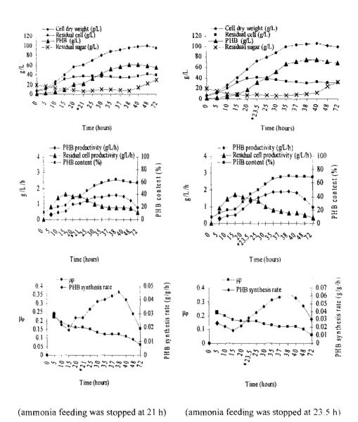
Fig.(2): Growth of A.latus ATCC 29712 and PHB production during 72 h incubation at 30°C on med.3 under nitrogen limitation condition (ammonia feeding was stopped at 21 h & 23.5 h) using bioreactor as a pH-stat fed-batch culture ( $\mu_p$ =specific production rate).
