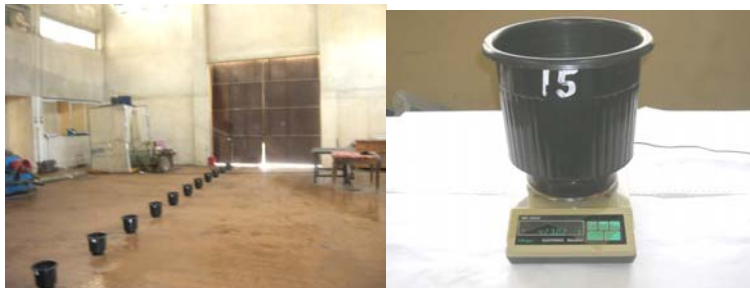
Figure (1): The water collector during the precipitation event Figure (2): weighting the water collector after the precipitation event
