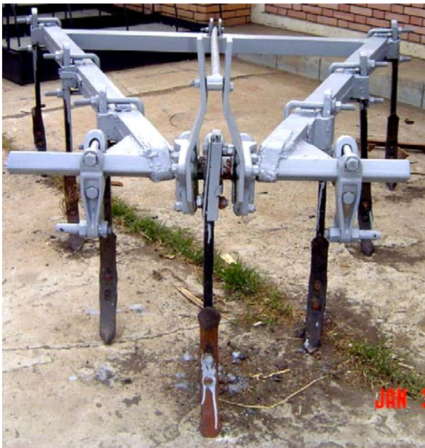
Fig. (2): Modified \Delta -shape chisel plow (4 rows).
