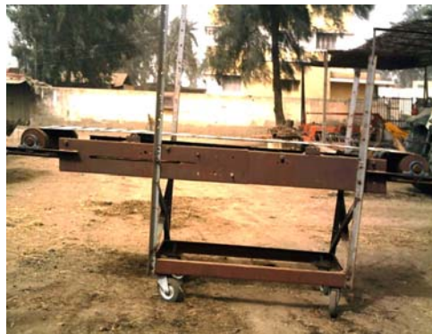
Fig. (3) Photo of the proposed belt conveyor.
