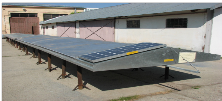
Fig. 3: Solar tunnel dryer in experimental place
