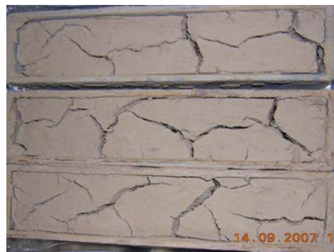
Fig. 8: Shrinkage and cracks for clay samples.
