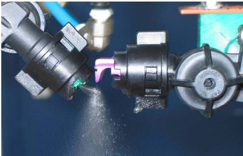
Fig. 4: Illustrates the combination of a tongue nozzle (Lechler FT5.0) for the air and a LU 110-015 for the liquid.
