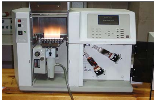
Fig. (2): Atomic Absorption Spectrophotometer (Varian, SpectrAA 55)
