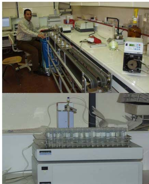
Fig. 5: Display the laboratory facilities instruments (LS 30 Fluorescence Spectrometer) to measure the spray deposition from different atomizers.
