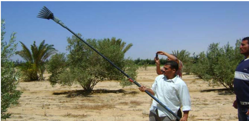
Fig.3: A vibrating comb harvesting model during field experiments
