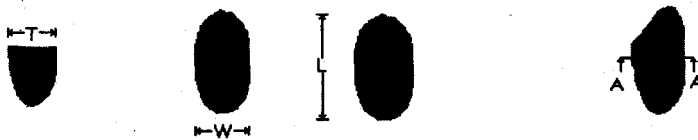
T = Thickness of largest section W= width of largest section L = Length of longest axis AA-The largest section perpendicular to the longest axis of kernel.
