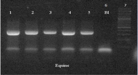
Lane 1, 2, 3, 4 and 5 shows Positive results of 5 representative samples (359 bp), Lane 6 shows result of a blank sample (359 bp) and Lane 7 shows the separation manner of 100 bp Marker.
