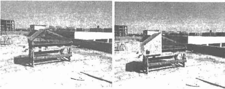
**Fig. (1): Asymmetrical double-slope solar still with and without shading.**
