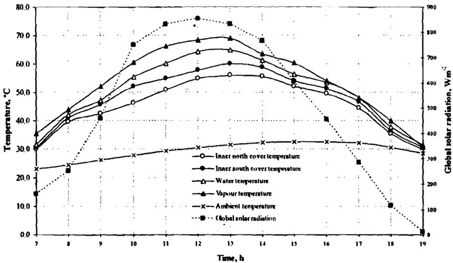
**Fig. (3): Solar intensity and temperature variations of different components of solar still with shading.**
