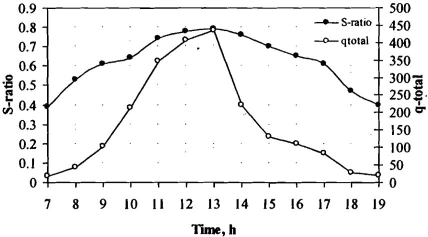
Fig. (9): Hourly average S-ratio between the evaporative heat transfer and the total heat transferred from the water to the cover.
