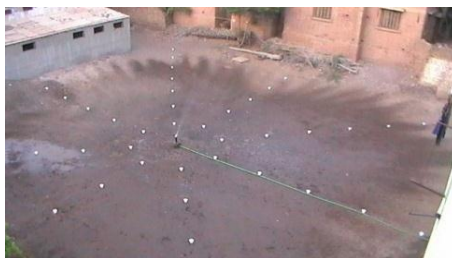
Fig. 15: The wetted pattern of MPS with first design by the internal nozzle dimensions (3x8.1) mm and closed valve
