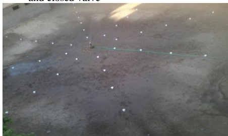
Fig. 19: The wetted pattern of MPS with first design by the internal nozzle dimensions (1x8.1) mm and closed valve
