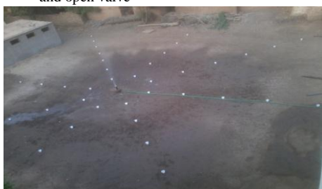
Fig. 18: The wetted pattern of MPS with first design by the internal nozzle dimensions (1x8.1) mm and open valve
