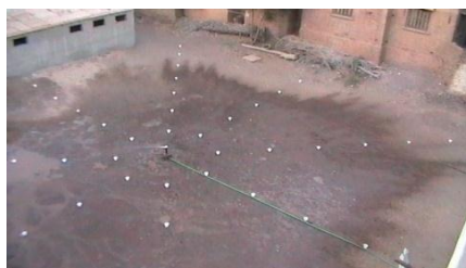
Fig. 24: The wetted pattern of MPS with second design by the internal nozzle dimensions ( 3 \times 11.8 ) mm and closed valve
