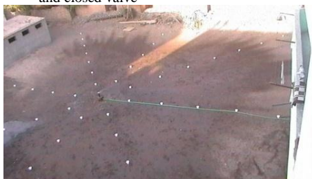
Fig. 17: The wetted pattern of MPS with first design by the internal nozzle dimensions (2x8.1) mm and closed valve
