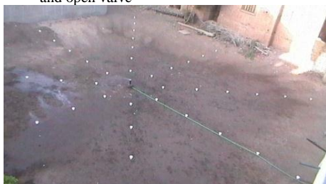
Fig. 16: The wetted pattern of MPS with first design by the internal nozzle dimensions (2x8.1) mm and open valve
