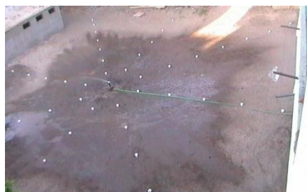
Fig. 23: The wetted pattern of MPS with second design by the internal nozzle dimensions ( 3 \times 11.8 ) mm and open valve
