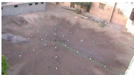
Fig. 14: The wetted pattern of MPS with first design by the internal nozzle dimensions (3x8.1) mm and open valve
