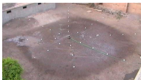
Fig. 26: The wetted pattern of MPS with second design by the internal nozzle dimensions ( 2 \times 11.8 ) mm and closed valve
