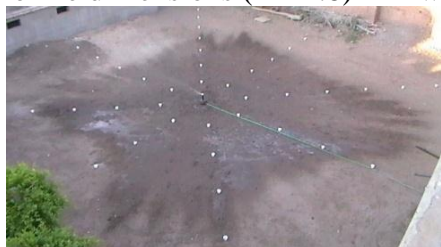
Fig. 21: The wetted pattern of MPS with second design by the internal nozzle dimensions ( 4 \times 11.8 ) mm and open valve
