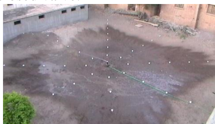
Fig. 22: The wetted pattern of MPS with second design by the internal nozzle dimensions ( 4 \times 11.8 ) mm and closed valve
