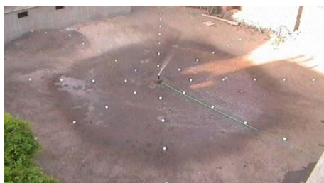
Fig. 25: The wetted pattern of MPS with second design by the internal nozzle dimensions ( 2 \times 11.8 ) mm and open valve
