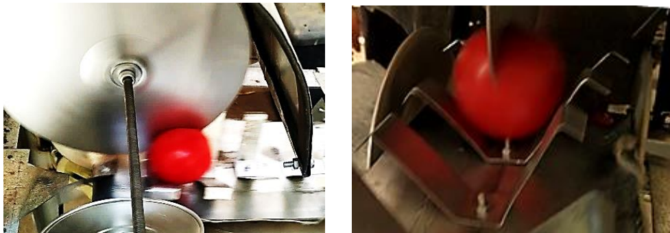
Figure (5): Processing of dividing tomatoes through operating of cutting unit
