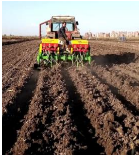
Figure (1): A new machine is used to prepare the soil for raised bed planting obtained from ICARDA project to help farmers in improving wheat cultivation in Egypt.
