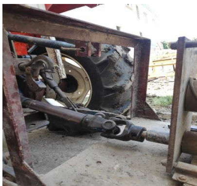
Fig. 3. Connection between tractor and the winch by flexible coupling
