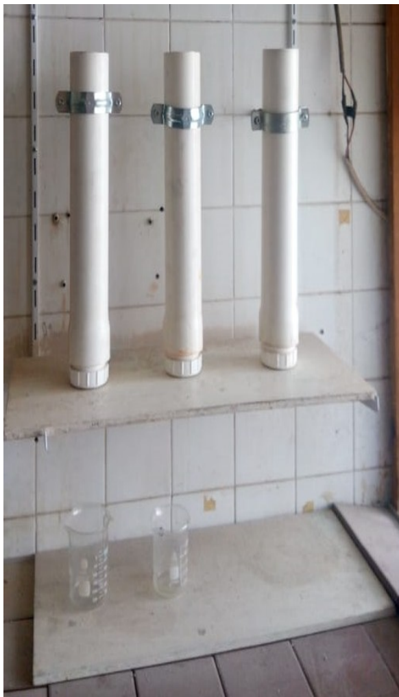
Fig. 1. Column experimental outline for the extraction of PTEs by citric acid (10 g L -1 ).
