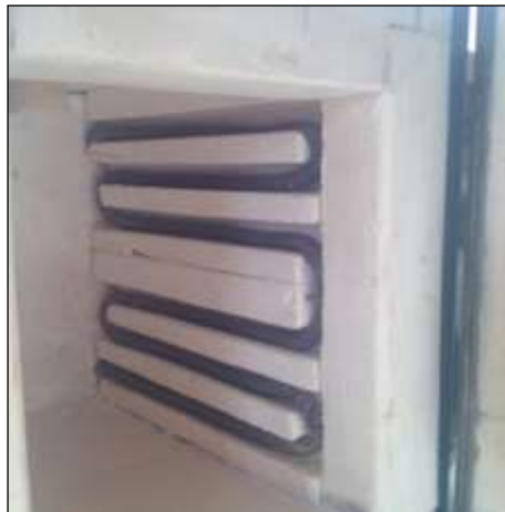
Fig. 13. The heating wire supported in the furnace lining grooves.
