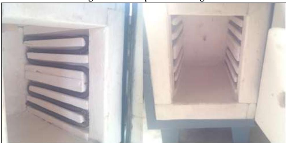
Fig. 10. Lining grooves for electric wire.
