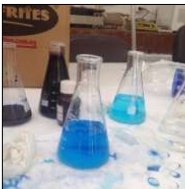
Fig. 27. Preparation the pyrolyzed samples to determine the adsorption by methylene blue test.
