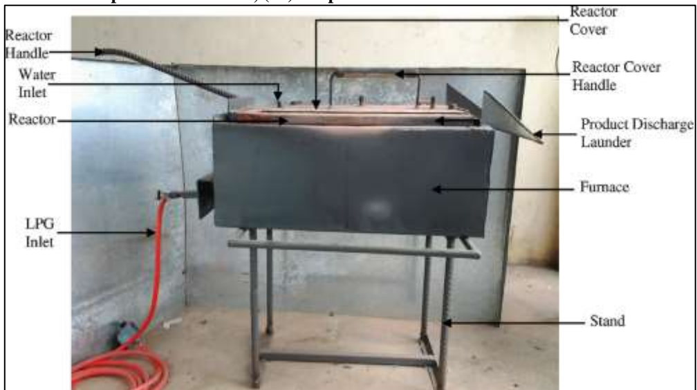
Fig. 3. Gasification/Activation Reactor System. (Buah and Kuma, 2016).
