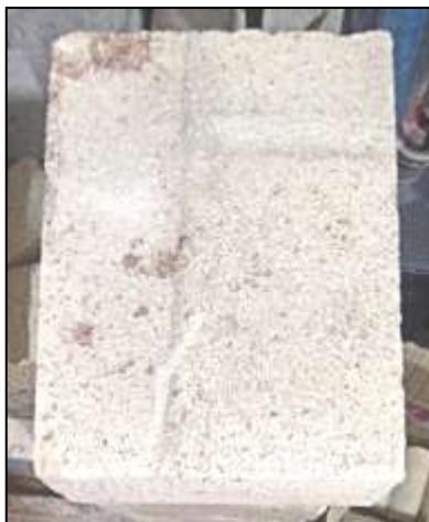
Fig. 9. Refractory used in lining.
