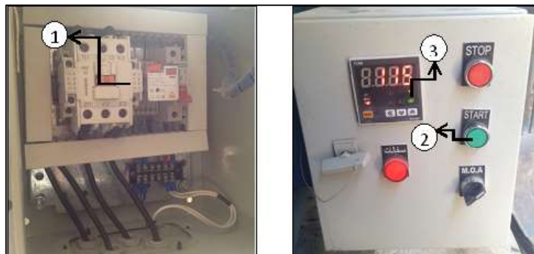
(a) The controller components. (b) The connection between furnace and controller.
