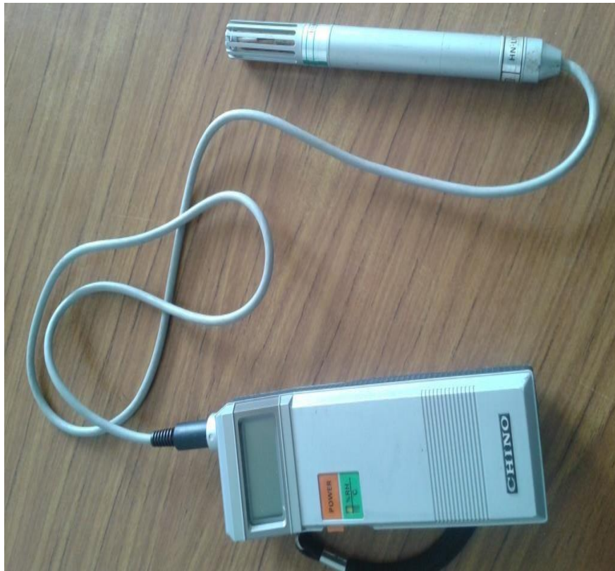
Figure 17. A digital air temperature and relative humidity meter
