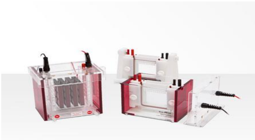
Figure (11): Biometra co-Mini electrophoresis system, 110 voltage, 120 amber, time taken: 2 hrs, Coomassie blue stain.
